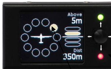
The direction of the impacting glider is marked with a **yellow big dot** on the display and the **red LED** becomes active (flashing).
