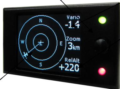
Selection is visualized with the **line** which is connecting the centre of the display and the glider symbol. If the near glider is also a member of the list of customized gliders, its ID will appear in the upper-left corner.
