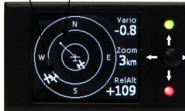
The green LED describes the GPS status of the Flarm unit: flashing means GPS status is bad. The red LED is active exclusively during warning status.
